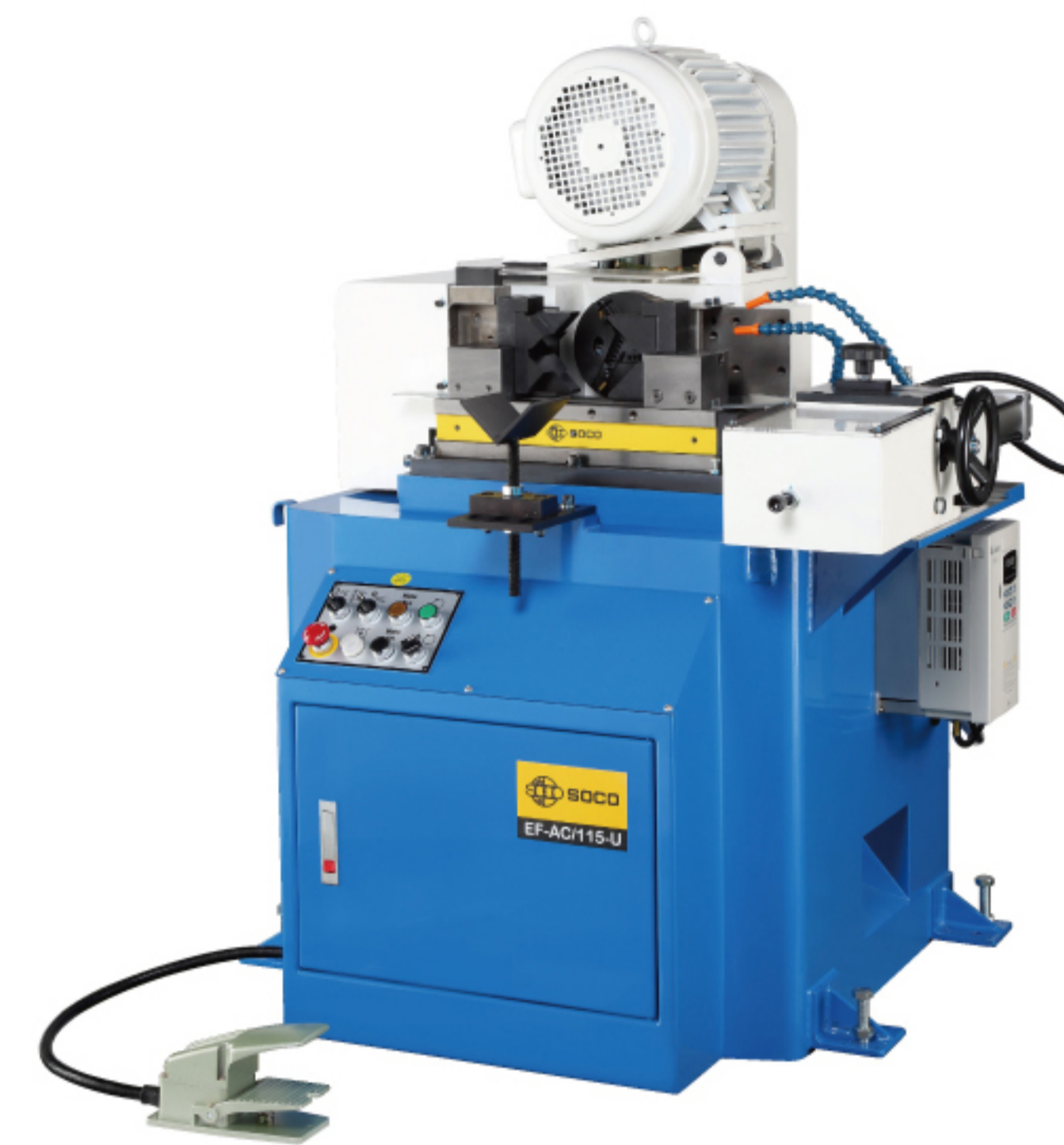
EF-AC/115-U Single tube end chamfering with Ø115mm capacity and equipped with a universal clamping
