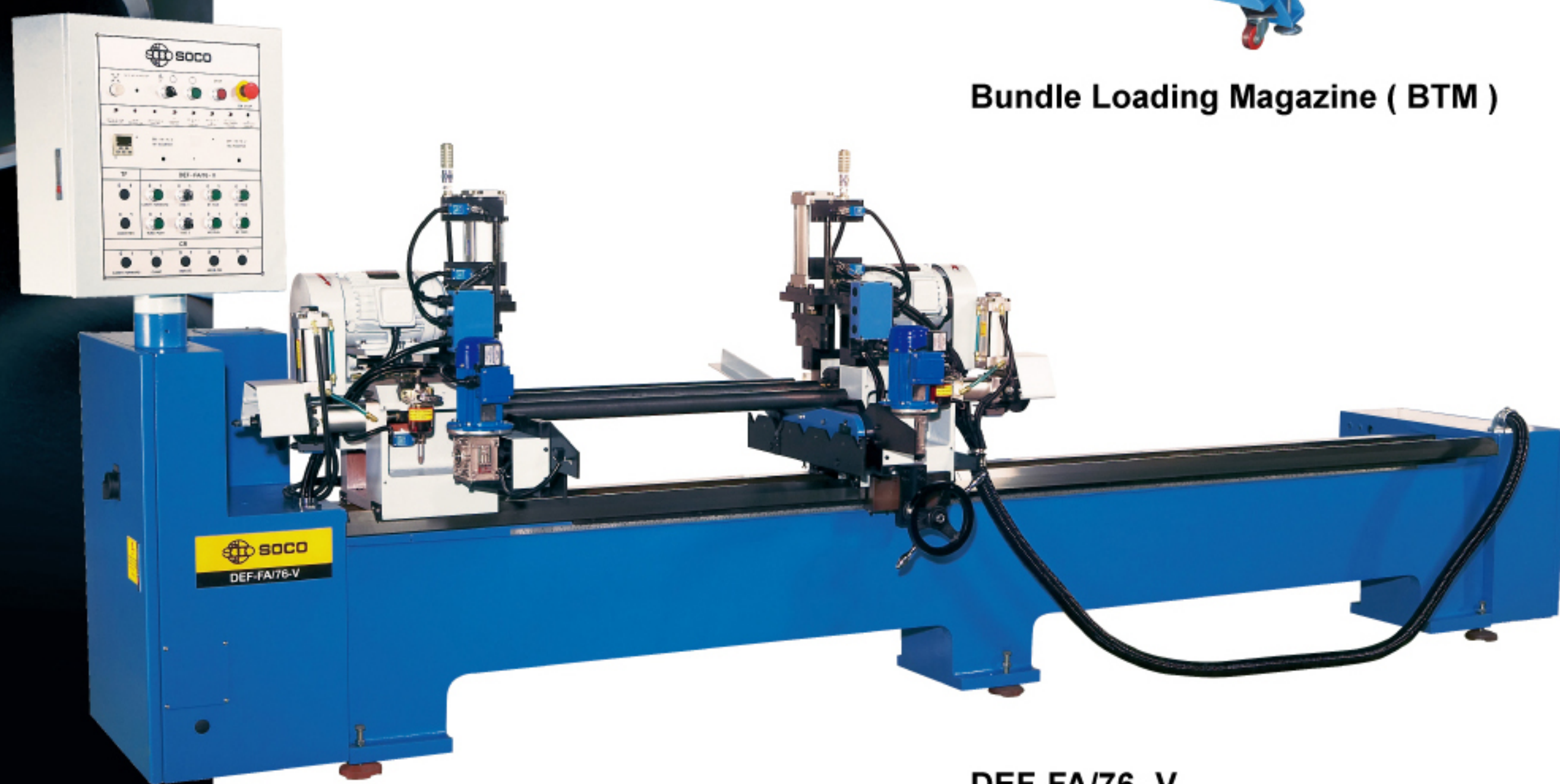
DEF-FA/76- V Double Tube Ends Chamfering with Long Working Lengths from 200mm ~ 3000mm. Capacity up to Ø76mm. Automatic Loading, Feeding and Chamfering. May connected to the SA-78NCE be an Automation Cells.
